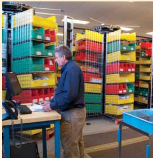
At Children's Hospital Colorado, horizontal carousels are used to pick thousands of pieces every day for use in the hospital.
